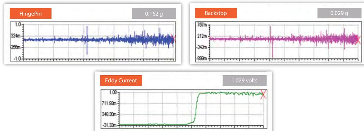
Figure 2 below is an example of acoustics being used properly in conjunction with a “look” technology. Eddy current indicates the disc is traveling from an open position to a close position upon cessation of flow. In this case, acoustics show the seating impact in the first 2 graphs, which is confirmed with the eddy current results in the same time domain.
